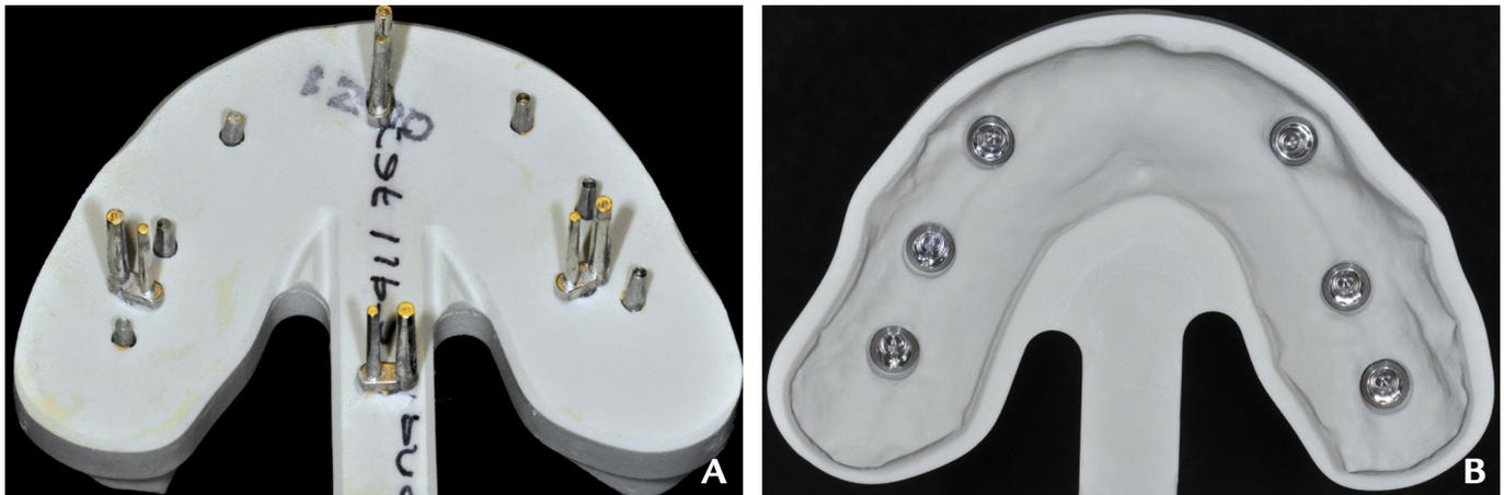
**2** A, Four dowel pins attached to base of definitive cast. B, Milled polyurethane definitive cast with removable implant analogs in place.
